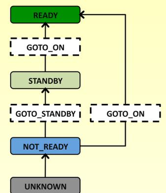
Figure on the right shows state diagram for the Tile Cal detector, where dashed lined boxes correspond to the implemented commands and the colored boxes represent allowed states. The arrows indicate allowed transitions between states.
