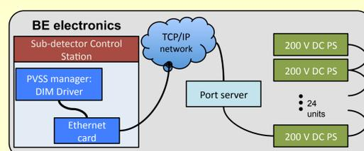
The Mod bus communication is established through the TCP/IP network, via the Port Server. The schematics of used Mod Bus readout chain is
