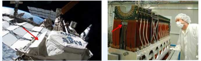
The AMS with the CO 2 cooling radiators visible (left) and LHCb-Velo with the CO 2 cooling evaporators (right)
